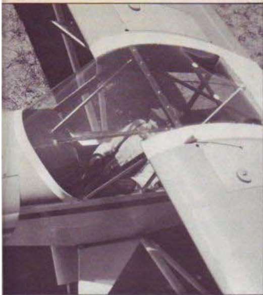
The Piper Super Cub used by the Air Force Academy to tow gliders has had a window modification to allow more visibility under critical towing conditions. The large 1/3 scale model also copied this conversion.
